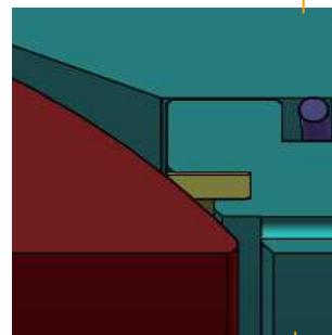
DPE VALVE: Single valve with two seating surfaces, each of which, in the closed position, provides a seal against pressure from a single source.
